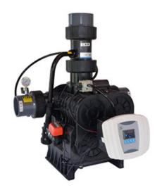
Material: The valve body is made of ABS plastic reinforced with 10% glass fibre, ensuring it is high impact resistant, heat resistant, and flame retardant. The valve core is made of a wear and corrosion resistant ceramic disc with a long service life and easy replacement.
