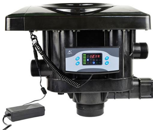
**Material:** The valve body is made of ABS plastic reinforced with 10% glass fibre, ensuring it is high impact resistant, heat resistant, and flame retardant. The valve core is made of a wear and corrosion resistant ceramic disc with a long service life and easy replacement.
