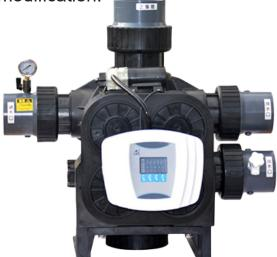
Material: The valve body is made of ABS plastic reinforced with 10% glass fibre, ensuring it is high impact resistant, heat resistant, and flame retardant. The valve core is made of a wear and corrosion resistant ceramic disc with a long service life and easy replacement.
