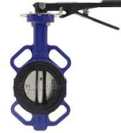
*Body: Ductile Iron, Disc: SS304, Stem: SS304, Seat: EPDM, Pressure: PN16*
